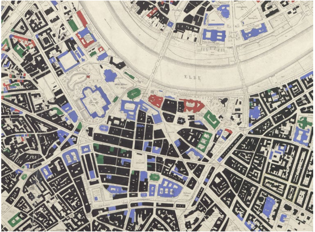
↑ Fig. 2. Dresden City Council, damage plan of the air raids in 1944/1945, Legend: black = completely destroyed, blue = heavily damaged, green = moderately damaged, red = slightly damaged (Stadtarchiv Dresden, StAD, Stadtbauamt 4.1.9, Dezernat Aufbau, Mappe 513)
